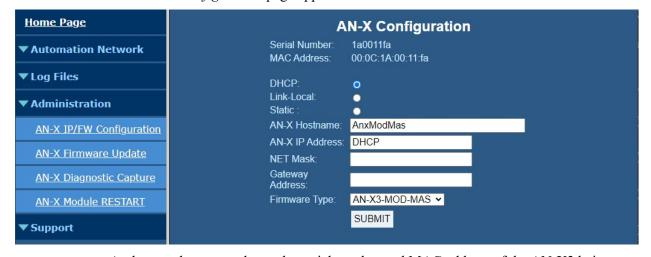
At the top, the screen shows the serial number and MAC address of the AN-X3 being configured.
